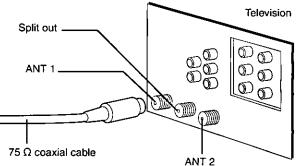
Connect to one of the terminals, then change the television's setting as necessary.
